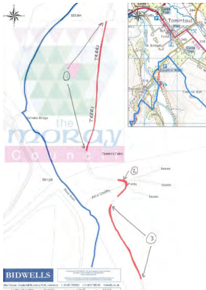
Fig. 3 : Location of maintenance works on existing track
